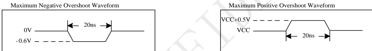
Figure 5-1 Maximum Overshoot Waveform
